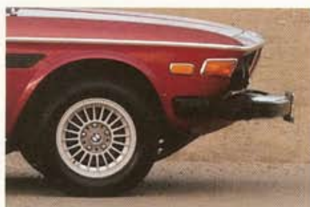
Five-mph impact bumpers appeared in 1974. Ugly, yes, but they've saved more than one front end. When hit, they collapse and are hard to repair.
